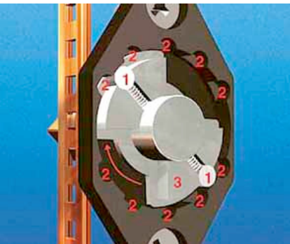
As the handle is turned, the security bolts (1) are carried by the coupling element (3) to the individual notches (2) producing the clicking sound.
