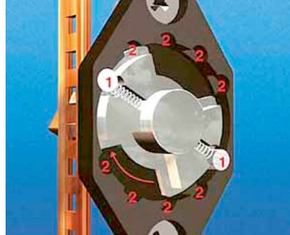
As the window handle is turned, the sprung security bolts (1) click as they go over special notches (2) in the housing, -indicating the built-in security
