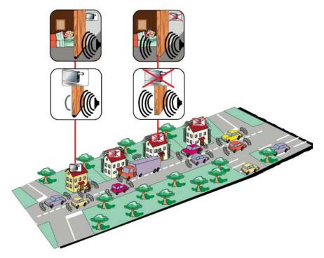
The sound insulation of a door bottom seal is measured in decibel according to ISO 140 and ISO 717 international standards.
