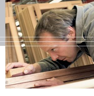
The Cetol WP 575 sanding sealer primarily serves the wood preparation to visually improve the subsequent coating quality. All water-soluble and/or solvent borne Sikkens Joinery paint and varnish systems can be used on the precision ground wood surface pre-treated in this way.
